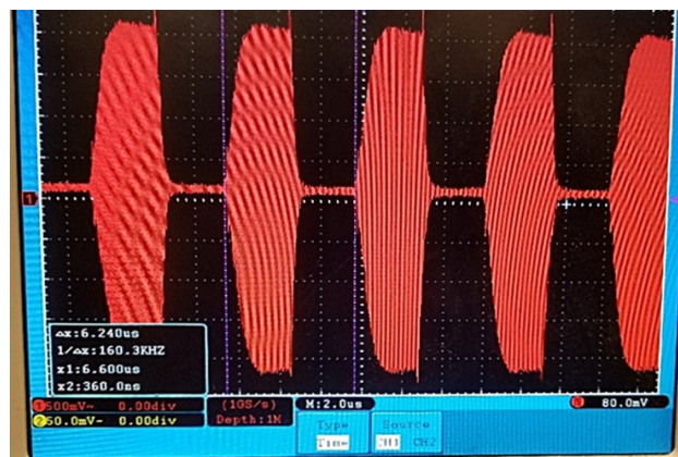
Pulse Output of Plasma Tube at 160 kHz, 50 % Duty Cycle
